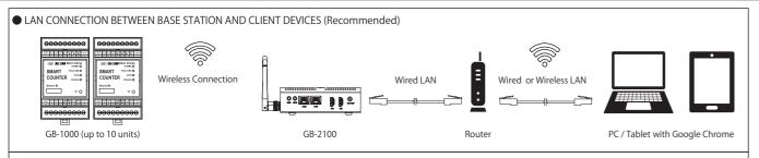
WIRELESS CONNECTION BETWEEN BASE STATION AND CLIENT DEVICES
