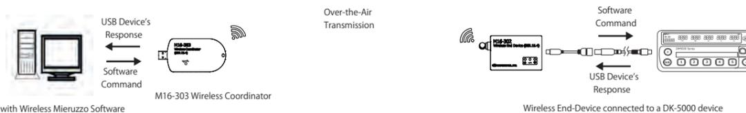
The wireless system operates at 2.4 GHz, employing IEEE 802.15.4 protocol. Up to 14 Wireless End-Device (M16-302 or M16-602) can be connected to the Coordinator device but only one end-device will be paired with the communication software at a certain time. Selection of end-device to be accessed can be done thru the software.
